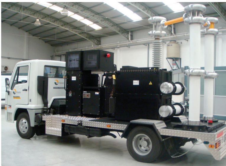
200kV VLF Withstand, VLF TD & VLF PD Test Truck Inducor Ingenieria S.A. Argentina
