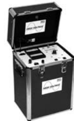
28 kV @ 1 μF @ 0.1 Hz
