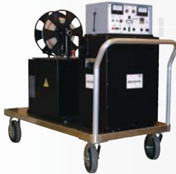
VLF-65CMF 0-65kV peak - sine wave 0.1 Hz @ 2.2 μF – 0.01 Hz @ 22 μF These two models are higher in power to test cables over 10 miles (16 km) long.
