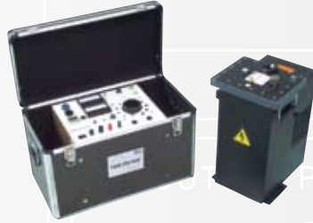
5 – 35 kV Cable Testing VLF-6022CM 0-60kV peak - sine wave 0.1 Hz – 0.02 Hz 1.1 μF – 5.5 μF
