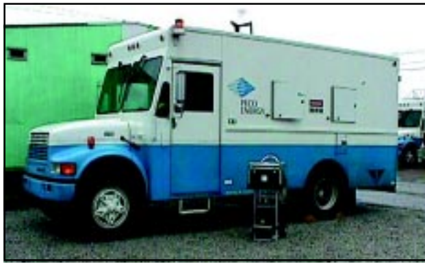
Fig. 2. A very low frequency 60-kV hipot set on a handcart sits next to a PECO Energy 60-Hz cable fault locating/hipot truck.
